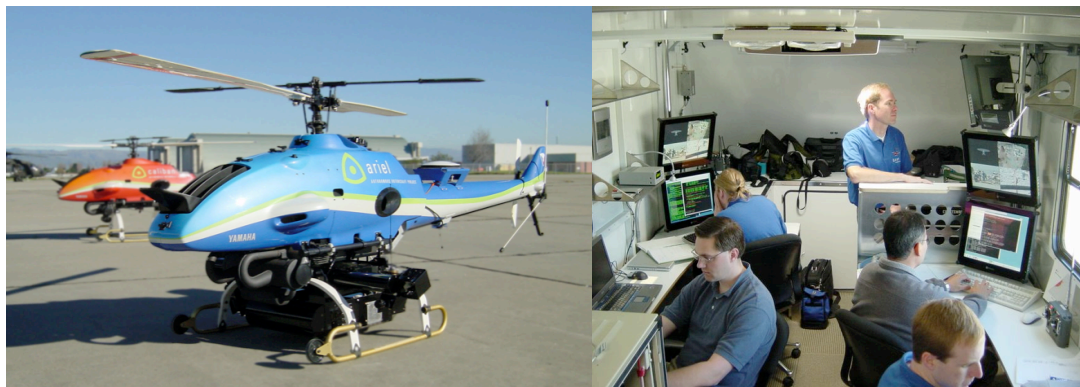
Figure 2: ARP RMAX research aircraft (left) and instrumentation trailer (right)
